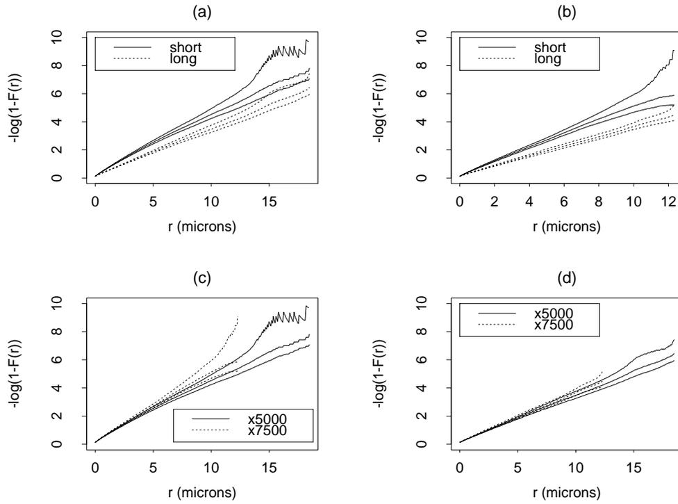
Fig. 7. Plot of  $-\log(1 - \hat{F}^{km}(r))$  against  $r$ , for the pooled Kaplan-Meier estimator. (a) The estimators for short and long heat treatment for magnification  $\times 5000$ ; (b) The estimators for short and long heat treatment for magnification  $\times 7500$ ; (c) The estimators for  $\times 5000$  and  $\times 7500$  for short heat treatment; (d) The estimators for  $\times 5000$  and  $\times 7500$  for long heat treatment.
