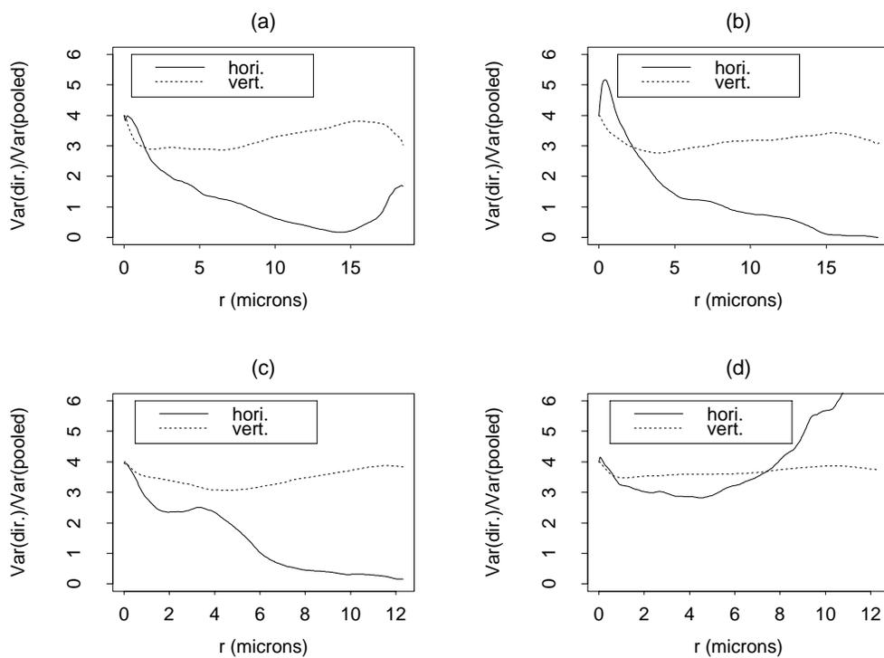
Fig. 5. Ratio of the estimated variance of the Kaplan-Meier estimator in horizontal and vertical directions to the estimated variance of the pooled estimator. (a)  $\times 5000$ , short; (b)  $\times 5000$ , long; (c)  $\times 7500$ , short; (d)  $\times 7500$ , long.
