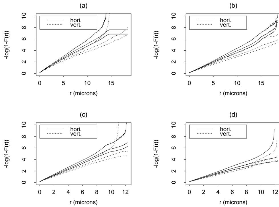
Fig. 4. Plot of  $-\log(1-\hat{F}^{km}(r))$  against  $r$ , for the pooled Kaplan-Meier estimator in horizontal and vertical directions. (a)  $\times 5000$ , short; (b)  $\times 5000$ , long; (c)  $\times 7500$ , short; (d)  $\times 7500$ , long.
