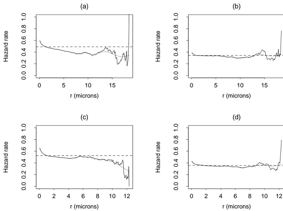
Fig. 10. Estimated linear contact hazard for the pooled estimates shown in Fig. 7. (a)  $\times 5000$ , short; (b)  $\times 5000$ , long; (c)  $\times 7500$ , short; (d)  $\times 7500$ , long. —: Point estimate;  $\cdots$ : Kernel smoothed function, see text; - - -: Hazard rate for the estimated Boolean model, see text.
