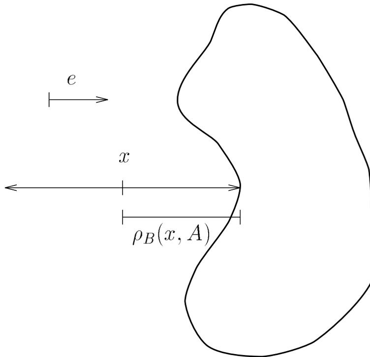
Fig. 2. In the text we have defined  $\rho_B(x, A)$  to be the "shortest" distance to  $A$  from  $x$  "looking in both ways" along the directional vector  $e$ .
