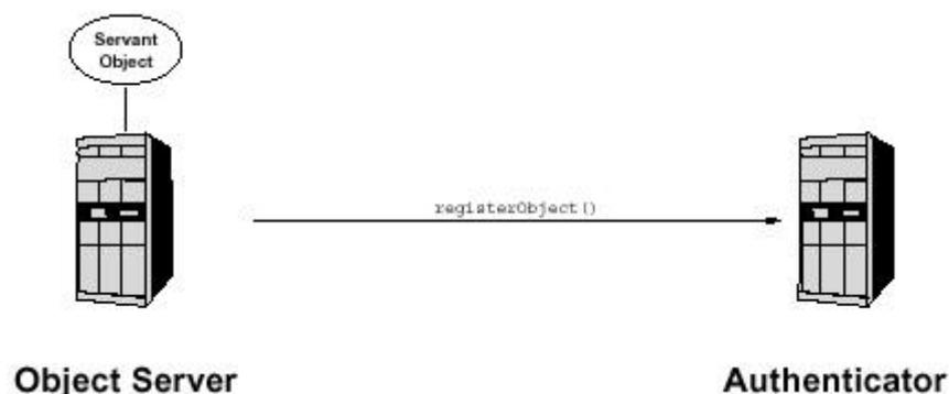
Figure 21 Registration of a servant object.
