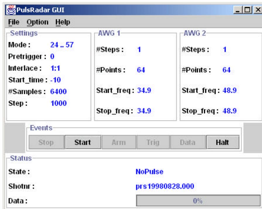
Figure 34 GUI for controlling the Pulsed Radar Reflector, either locally or remotely.
