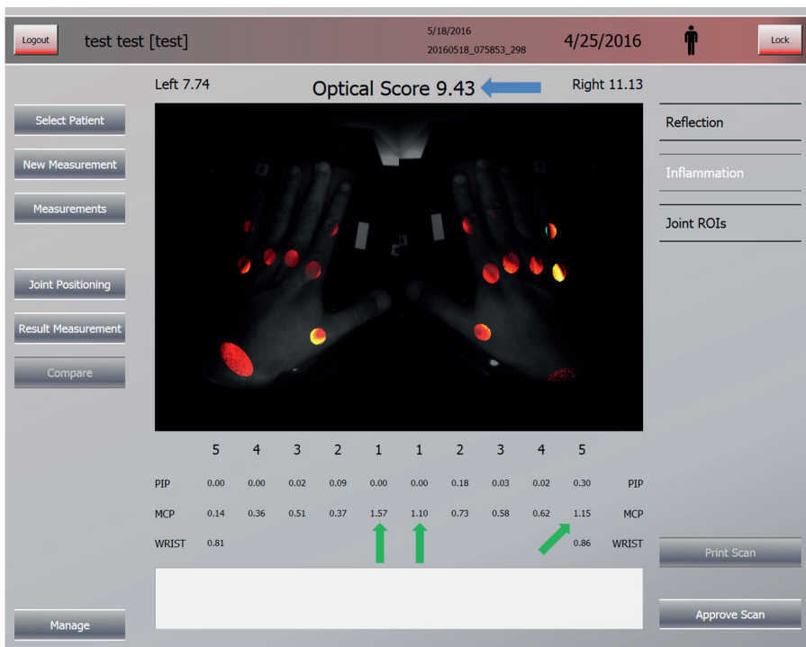
Figure 2: The HandScan user interface; total and individual optical joint scores. The total optical joint score of 9.43 (blue arrow) meets the HandScan remission criterion for total score. Individual optical joint criteria are shown below the picture. There are three joints (green arrows) that exceed the individual optical joint score criterion ( >1 ). Regarding the HandScan remission criteria (total optical spectral transmission (OST) score \leq 11 AND a maximum of one joint with OST >1 ), this (test) patient is not in remission.
