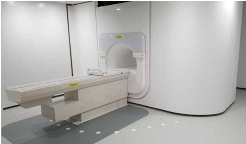
● Figure 2 Schematic design of the MRL (top), and the actual MRL constructed at UMC Utrecht (bottom). The MRL integrates a 1.5 T MRI scanner and a 7 MV photon linac, which is mounted on a ring-shaped rotating gantry.
