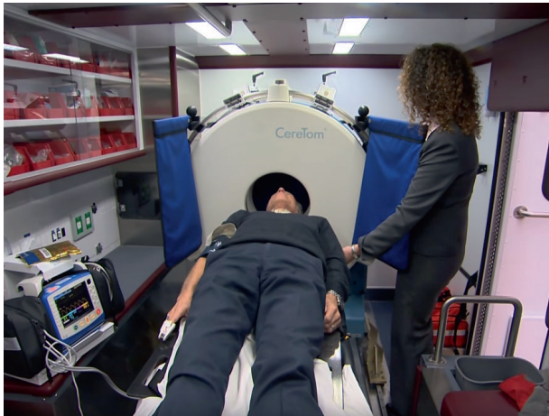
Fig. 7.4: A small-bore CT scanner inside a mobile stroke unit. The University of Texas Health Science Center takes the CT scanner to the patient by equipping an ambulance with a CereTom (Samsung NeuroLogica Corporation, Boston, USA).
