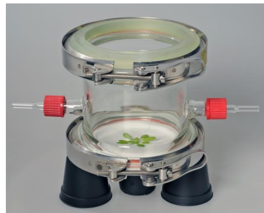
Figure 2.2 A four-week old Arabidopsis thaliana Col-0 plant in the small plant chamber with the lid with quartz glass. The pot in the middle contains plant roots and soil, pots on either side are for support.
