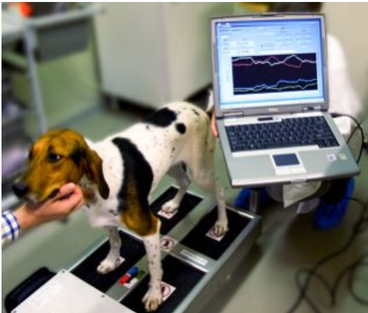
The four-plates balance (4PB) in the animal laboratory facility. The dog is standing freely. In case of major movement within the 10 seconds, the measurement was started over.
