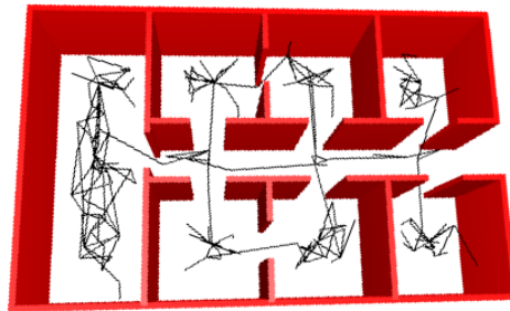
Figure 13: A roadmap that is collision-free with respect to the static obstacles. The rotational degrees of freedom are not shown in the roadmap.
